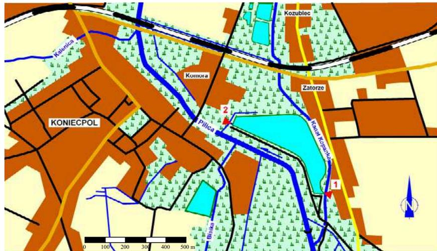
Fig. 2. Location of measurement-control points on the inflow to (1) and outflow (2) from the reservoir
