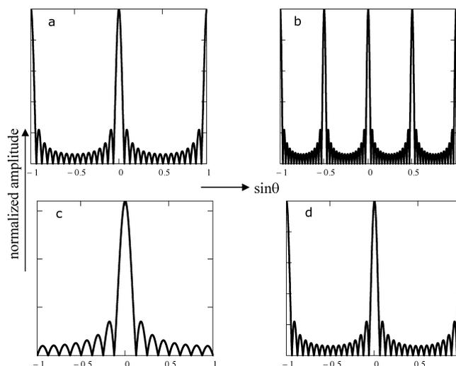
Fig. 5. The transmit/receive far field beam pattern for 8 elements array, a) phase array,  $d = 1.2\lambda$ , b) SAF,  $d = 1.2\lambda$ , c) phase array  $d = 0.5\lambda$ , d) SAF,  $d = 0.5\lambda$ . The distance between grating lobes for SAF two times shorter (Eq. (15)) than for the phase array beam forming.
