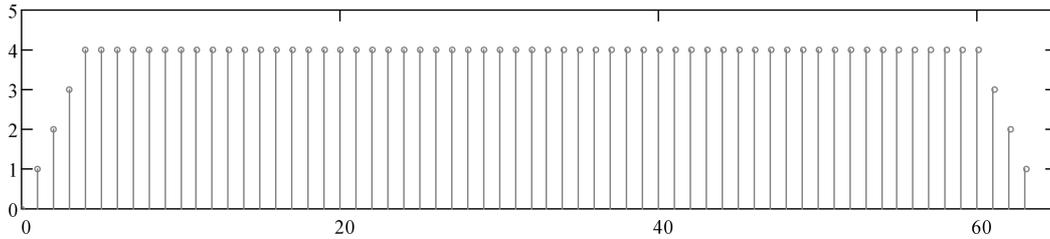
Fig. 7. Effective aperture of 32 elements M-SAF and  $K_T = K_R = 4$  shifted by full length of subapertures (four elements).
