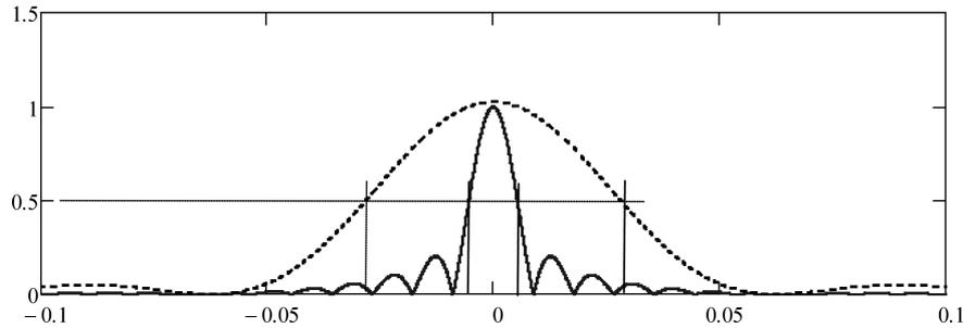
Fig. 8. Far field response for 32 elements; solid line M-SAF with  $K_T = K_R = 4$  shifted by full length of subapertures (four elements), dashed line – phase array. Lateral resolution for M-SAF is roughly 5 times better.
