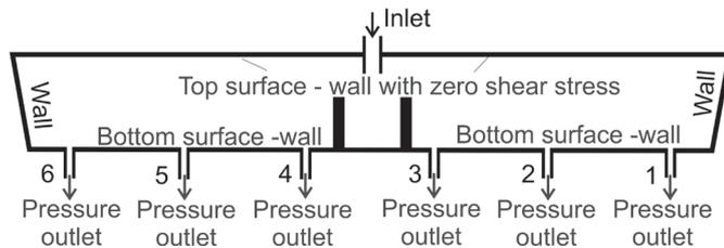
Fig. 2. Boundary conditions set for numerical simulations
