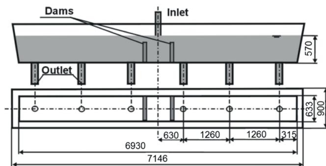
Fig. 1. Characteristic dimensions of the investigated tundish [12]
