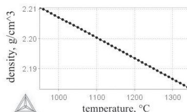
Fig. 1. Dependency of graphite's density on temperature
