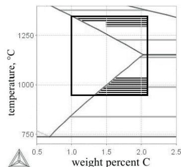
Fig. 6. Fragment of Fe-C phase diagram, field inside marked rectangle indicates considered in calculations range of temperature and carbon concentration. Lined field marks zone with biggest error  $\Delta\rho$
