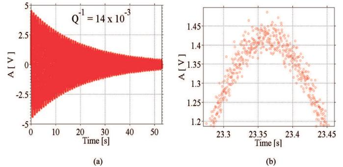
Fig. 2. (a) Illustration of exponentially damped harmonic oscillations with additive Gaussian noise for  $Q^{-1} = 0.014$ . (b) A part of the free decaying signal around a peak embedded in the experimental noise,  $S/N = 32$  dB. The resonant frequency  $f_0 = 1.12345$  Hz, the sampling frequency  $f_s = 3$  kHz
