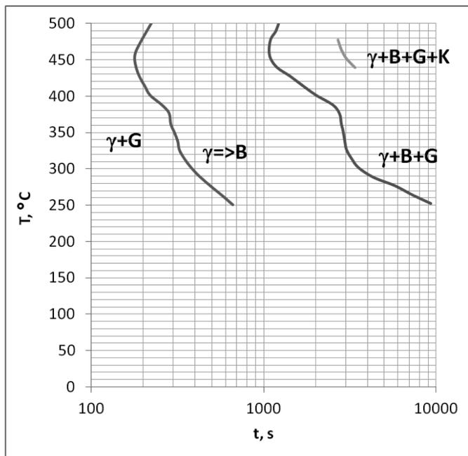
Fig. 3. TTT diagram for the ductile iron 1 after digitalization
