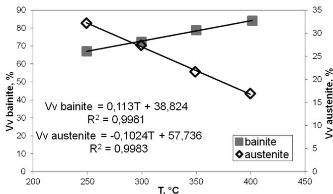
Fig. 5. The volume fraction of the retained austenite and of the bainite vs. the transformation temperature [10]
