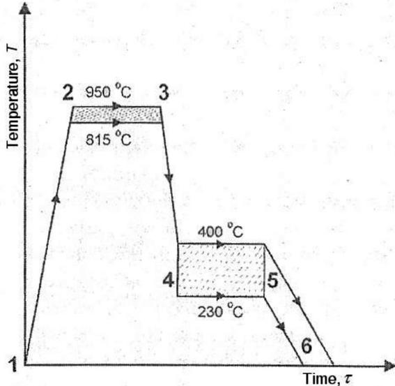
Fig. 1. Schematic illustration of all stages of austempering heat treatment [7]
